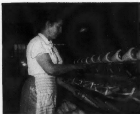
WINDER— Mrs. Turcotte winds single wool yarn from the spinning bobbin to a paper cone in order to make a long continuous strand of yarn. The yarn is later used as a supply package in doubling.
