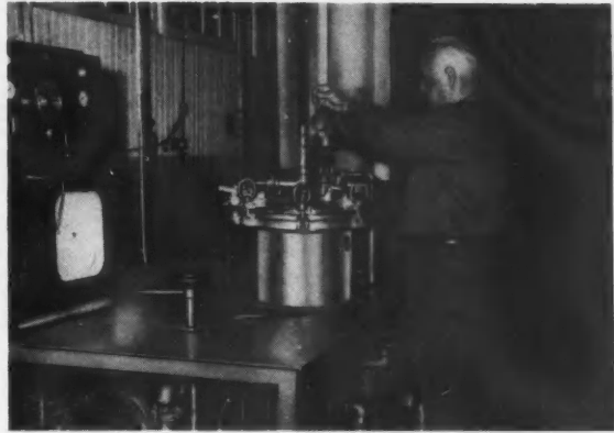
DYE JOB —McIntire at work during the first shift at Willimantic operating a Gaston County Pressure Dye machine—used for small dye lots of yarns that need special attention. Dye temperatures from 120° F to 250° F are used in the dye baths with a complete range of colors.
